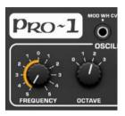
You modify parameters using rotary encoders by clicking on the button then moving the mouse cursor vertically up or down.
