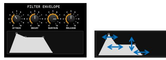
When moving the anchors, the corresponding ADSR encoders will also turn and the parameter name and value will be displayed in the screen of the top panel area.
